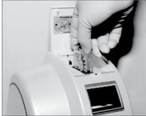
**NOTE :** Do not force the cartridge into the analyzer. The cartridge is designed to fit only in one way.
